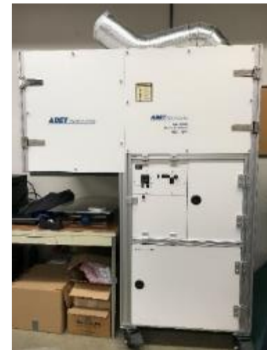
Solar Simulator -Abet Technologies Model 11048-1 3 kW multi-sun UV solar simulator, customer reconfigurable to a full spectrum 2 suns 300x300 mm field simulator.
