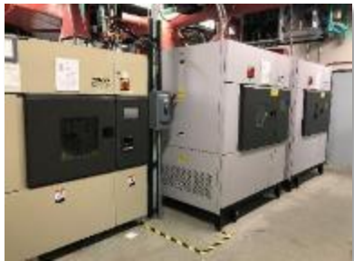
Ci5000 Weatherometer Xenon arc lamp exposure chamber-2 Suns, 60°C, 60 %RH
