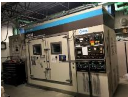
XR260 Weatherometer integrates the recent developments in environmental chamber and xenon solar simulation technology. The XR260 is capable of testing modules up to 1.9 meters by 1.4 meters.
